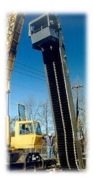
Due to the interlaced assembly of the filter elements on the belt shafts, the removed screenings are effectively ejected off the face of the belt as the belt follows the formed guides around the screen frame. As the belt enters the discharge area it becomes horizontal which allows for ease of discharge of the material. A rotary brush is also used in this area to minimize the opportunity for any carry over.
